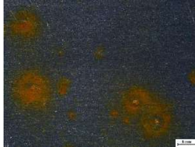
Figure 5. Crocin adsorbed on surface defects of 1050 specimen after immersion in the inhibiting solution for 13 weeks, as observed by Stereomicroscopy.
