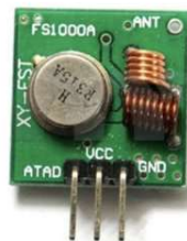
Sender modul: Pin 1: Data Pin 2: 5V VCC Pin 3: GND
