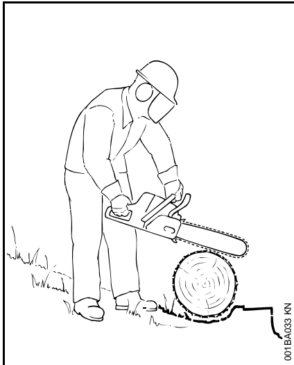
Bucking is cutting a log into sections.
