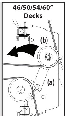
5. Use the deck lift pedal and deck lift knob to place the deck in the lowest position and use the multi-tool (a) to lock the deck lift components in place as shown in Figure 36.
