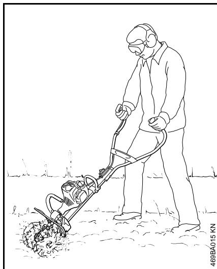
Cultivator MultiTools are available in versions with pick tines (BF-MM) and bolo tines (BK-MM).
