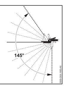
The angle of th cutter bar can be adjusted upwards in 4 stages from 0° (straight) to 55°, and downwards in 7 stages from 0° to 90° (right angle facing down). There are therefore 12 possible working positions.
