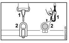
Press down the bar on the carabiner (1) and pull the carrying ring (2) out of the carabiner.
