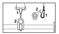
Attach the carabiner (1) to the carrying ring (2) on the drive tube – hold the carrying ring steady.
