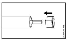
If the plug comes out of the drive tube when you pull off the cap:
