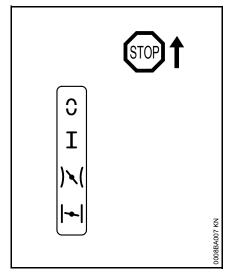
STOP or 0 – Master Control lever must be pushed in direction of STOP or 0 to switch off the ignition. When released, the Master Control lever springs back to the normal run position I and the ignition is switched on again.
