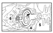
Squeeze grease into the gearbox housing (arrow) between the cam (4) and cutting blade (5) a little at a time (max. 5 g (1/5 oz)) while turning the drive pinion (6) with a hex key to distribute the grease evenly – avoid contact with the cutting blades.
