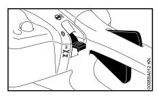
Press down the throttle trigger lockout and open the throttle – the Master Control lever moves to the
