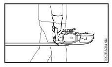
Carry the power tool by the handle – cutting blades behind you. Do not touch hot parts of the machine, especially the muffler and gear housing – **risk of burns!**
