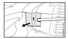
Carefully pry open the flap (1) with a suitable tool (e.g. combination wrench).
