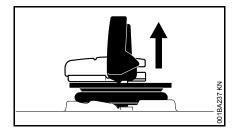
Remove the tank cap.
