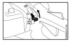
Move the Master Control lever in the direction of STOP or 0 – when released, the Master Control lever springs back to the normal run position I.
