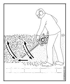
Swing the cutting blade from the bottom upwards in an arc – lower the nose of the blade, move along the hedge and then swing the blade up again in an arc.
