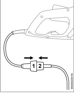
Insert the plug (1) into the extension cord coupling (2).
