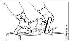
Push down the trigger switch lockout (2), depress the trigger switch (3) and hold them in that position.
