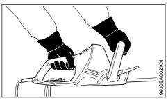
Left hand on the control handle and right hand on the loop handle.
