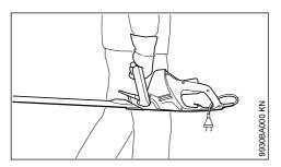
Carry the machine by the handle – with the cutting blades pointing to the rear.
