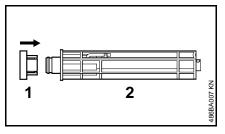
• Push the grass shield (1) onto the axle (2) as far as stop.
