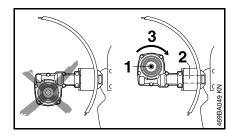
The axle (1) must be above the shaft (2). Direction of rotation (3) of MultiTool.
