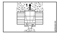
Guide the PowerSweep at right angles to the direction of travel (1).
