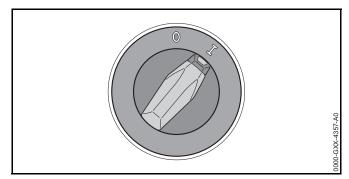
► Turn the rotary switch to the I position.
