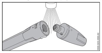
Flush nozzle and spray lance under running water and dry with a cloth.
