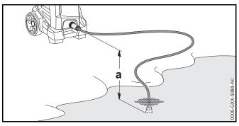
So that the water can be drawn in, the height difference between the pressure washer and the water source should not exceed the maximum suction lift (a), 19.1.
