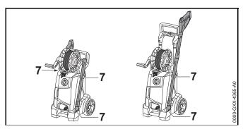
Store the spray attachment in the retainers (7) on the pressure washer.
