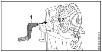
► Push the crank handle (1) into the recess (2). The crank handle (1) audibly engages.
