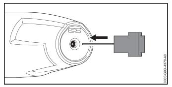
► If the nozzle is blocked up: Clean the nozzle with the cleaning pin.
