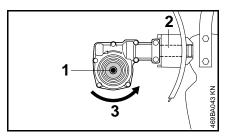
The axle (1) must be below the shaft (2). Direction of rotation (3) of MultiTool.
