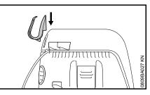
Attach holder for power cord on the right tab on the upper part of the vacuum cleaner
