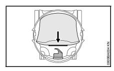
• Push filter bag sleeve onto intake port as far as possible
