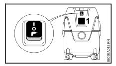
Power tools can be plugged into the machine socket (1). Do not exceed the maximum connected load of the machine socket – see "Specifications".
