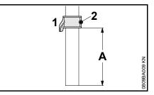
Slide the suction tube holder (1) via the suction tube (distance A approx. 8 cm / 3.150 in.) and secure it with the screw (2)
