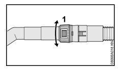
Turn adjusting ring (1) and adapt suction power to the relevant cleaning task
