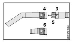
Slide clutch (3) of suction hose into the retainer (4) on the hand tube – lock (5) must engage When using the adapter for electric power tools (supplied with the model SE 62 E):
