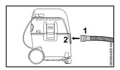
• Insert sleeve (1) of suction hose into the intake port (2)
