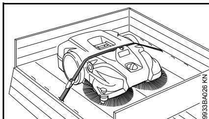
Use a strap to secure the machine in position.
