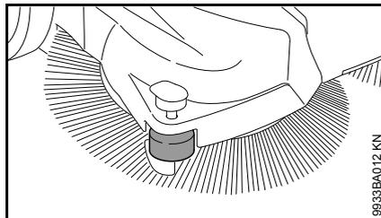
The guide roller makes it easier to control the sweeper along edges, e.g. next to walls or curbs.
