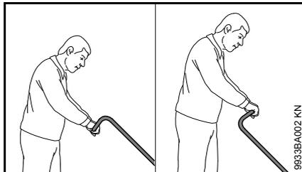
The push handle can be mounted in 2 different positions to suit the height of the user.
