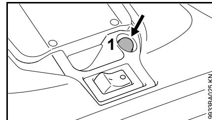
The thermal overload cutout for the side brooms resets automatically, while the overload cutout for the roller brush has to be reset manually by pressing the switch (1).
