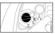
Choke knob automatically returns to the run position - when the throttle trigger is operated.
