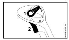
Infinitely variable throttle setting – throttle trigger can be locked in any required position: Move setting lever (1) upwards until required engine speed is reached. To disengage, move the setting lever back to the normal run position **I**.
