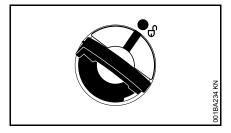
Marks on tank cap and fuel tank must line up.
