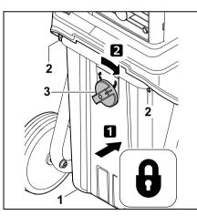
Insert shredder bag (1) at two guides (2) and push in as far as it will go. • Turn locking switch (3) to the right as far as it will go and secure the shredder bag.
