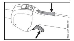
Press down the throttle trigger lockout and open the throttle – the choke knob moves to the run position **I**. After a cold start, warm up the engine by opening the throttle several times.
