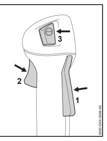
1 Throttle trigger lockout
