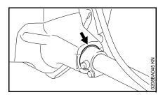
A vibration-absorbing rubber element is installed between the powerhead and the drive tube. Have it checked if there are signs of wear or a noticeable increase in vibration levels.
