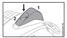
Fit cap (1), insert and tighten screw (2)
