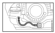
Check the pickup body in the fuel tank every year and have it replaced if necessary.
