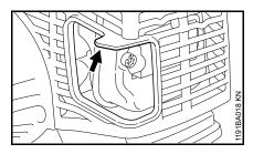
The spacer (arrow) is integrally molded to the shroud.
