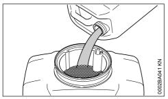
► Pour thoroughly mixed spray solution into the container through the strainer.
