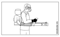
Carry the power tool on your back with both harness straps – do not hang it over one shoulder. Hold and control the blower tube with your right hand on the control handle – even if you are left-handed.
