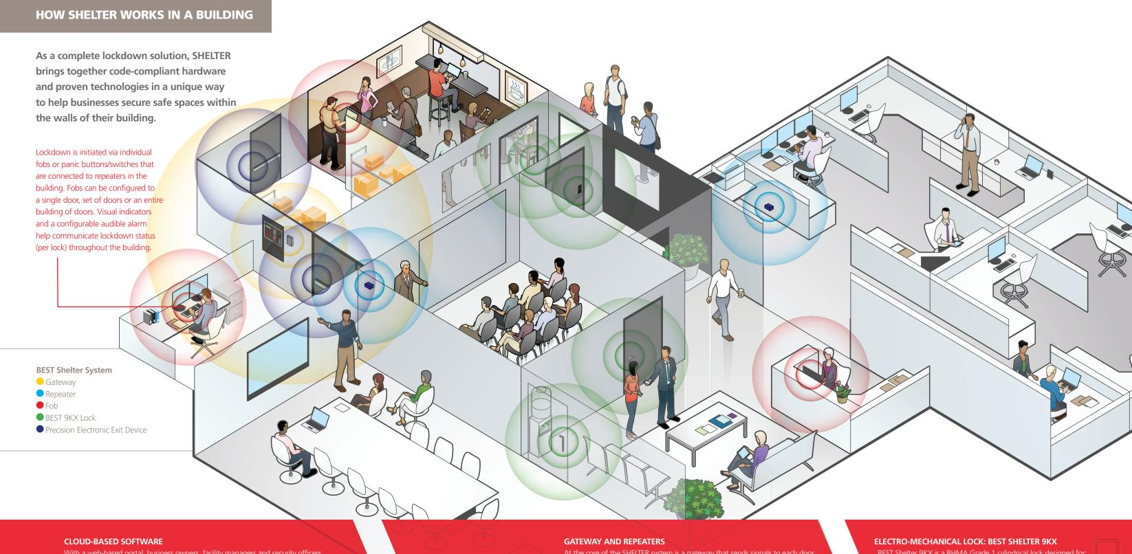
With a web-based portal, business owners, facility managers and security officers can configure the system from any web browser, wherever they are. The software allows you to configure a fob to lock down one door, an entire wing, or the whole facility. In addition, you can use the software to view self diagnostic test reports and send email/text notification for lock down status changes and self diagnostic results.
