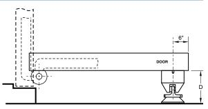
900 base has a minimum: 1-1/2" (38mm) extension. Maximum: 10" using combination of spacers [1/2" (13mm), 3/4" (19mm), etc.] Longer armature projections may encourage abuse and/or the weight of the extended rods will pull off the face of the door.
