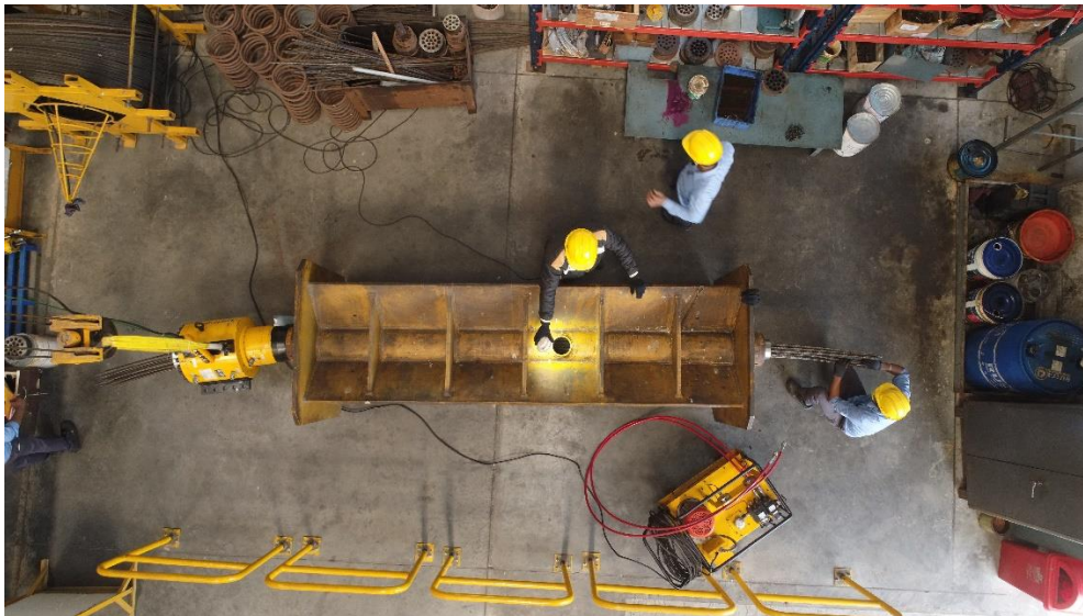
Anchorage Efficiency Testing Setup
