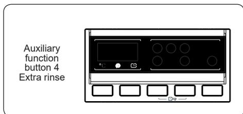
You can add an additional rinse operation to the end of the selected wash programme using this additional function.
