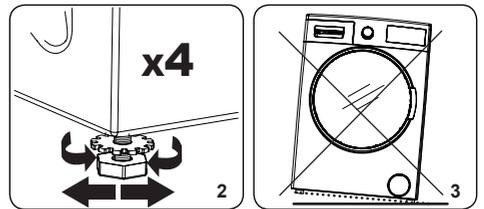
2. To increase the height of the machine, turn the feet clockwise. To decrease the height of the machine, turn the feet anticlockwise.
