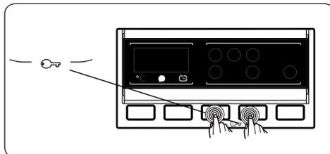
The Child Lock function allows you to lock the buttons so that the wash cycle you have chosen cannot be changed unintentionally.
