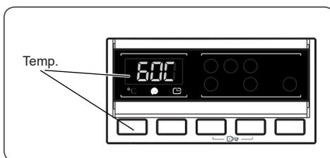
Use the washing water temperature adjustment button to alter the automatically programmed washing water temperature.
