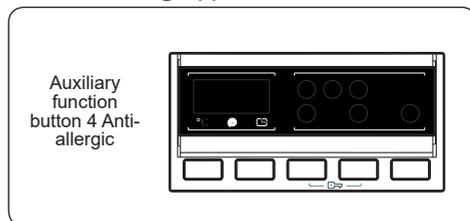
You can add an additional rinse operation to your laundry using this additional function. Your machine will carry out all rinsing steps with hot water. We recommend this setting for laundry worn on delicate skin, baby clothes and underwear.
