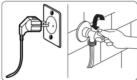
Turn your mains power supply off and remove the plug from the socket before carrying out maintenance and cleaning of your machine.
