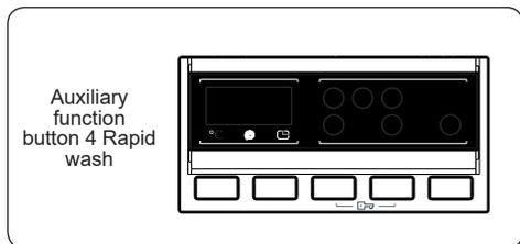
You can wash your laundry in a shorter time, using less energy and water by selecting this additional function.
