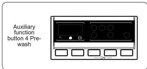
This additional function allows you to give heavily soiled laundry a pre-wash before the main washing programme takes place. When using this function, put detergent in front washing compartment of the detergent drawer.
