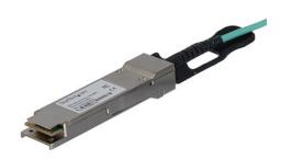
The QSFP40GAO7M is an MSA compliant optical quad small form-factor pluggable (QSFP+) cable that is designed, programmed and tested to work with 40 GbE compatible switches and routers. This AOC QSFP+ cable supports 40 Gigabit Ethernet applications (4 x 10GbE) connected through QSFP+ ports. It is a low-power, low-latency cable that is hot-swappable, making upgrades and replacements seamless by minimizing network disruptions.
