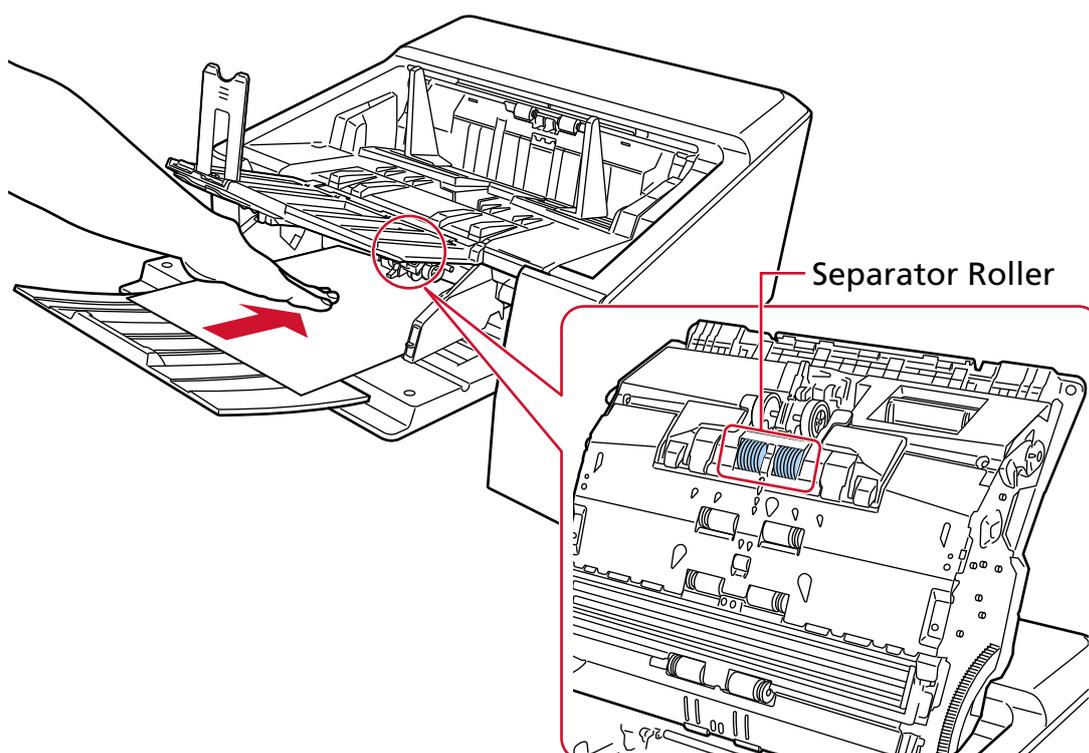
The document is picked, scanned, then ejected onto the stacker.
