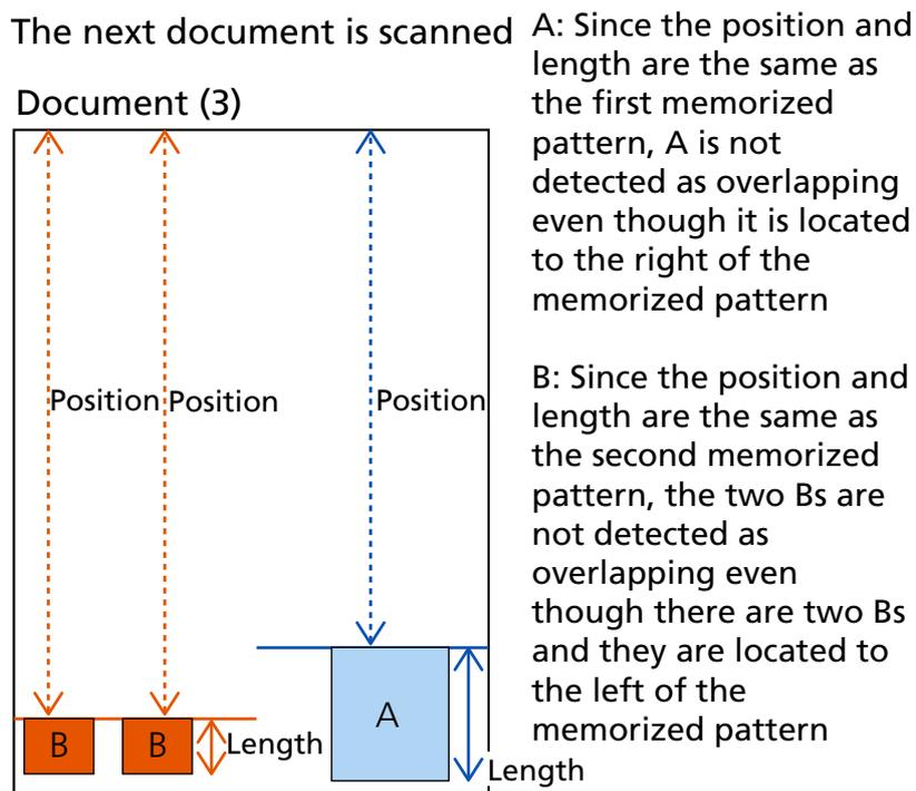
Overlap patterns can be memorized for up to 32 sheets (up to four overlap patterns can be memorized per sheet scanned).
