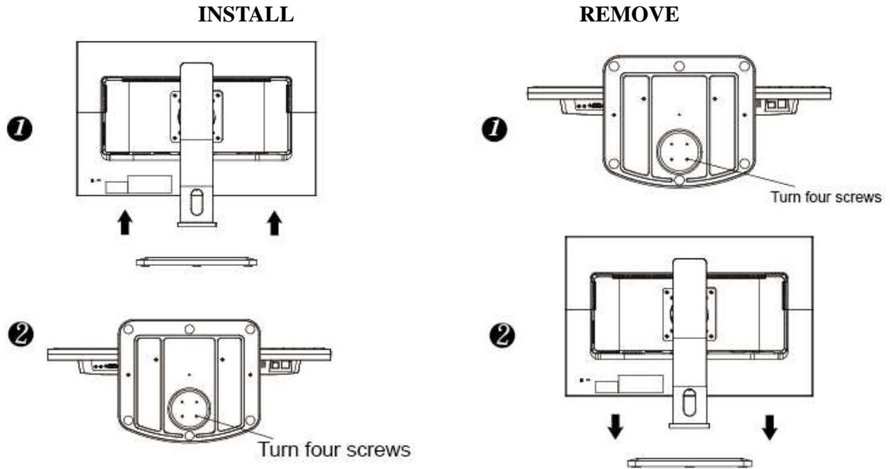
Figure.1. Installing and Removing the Base
