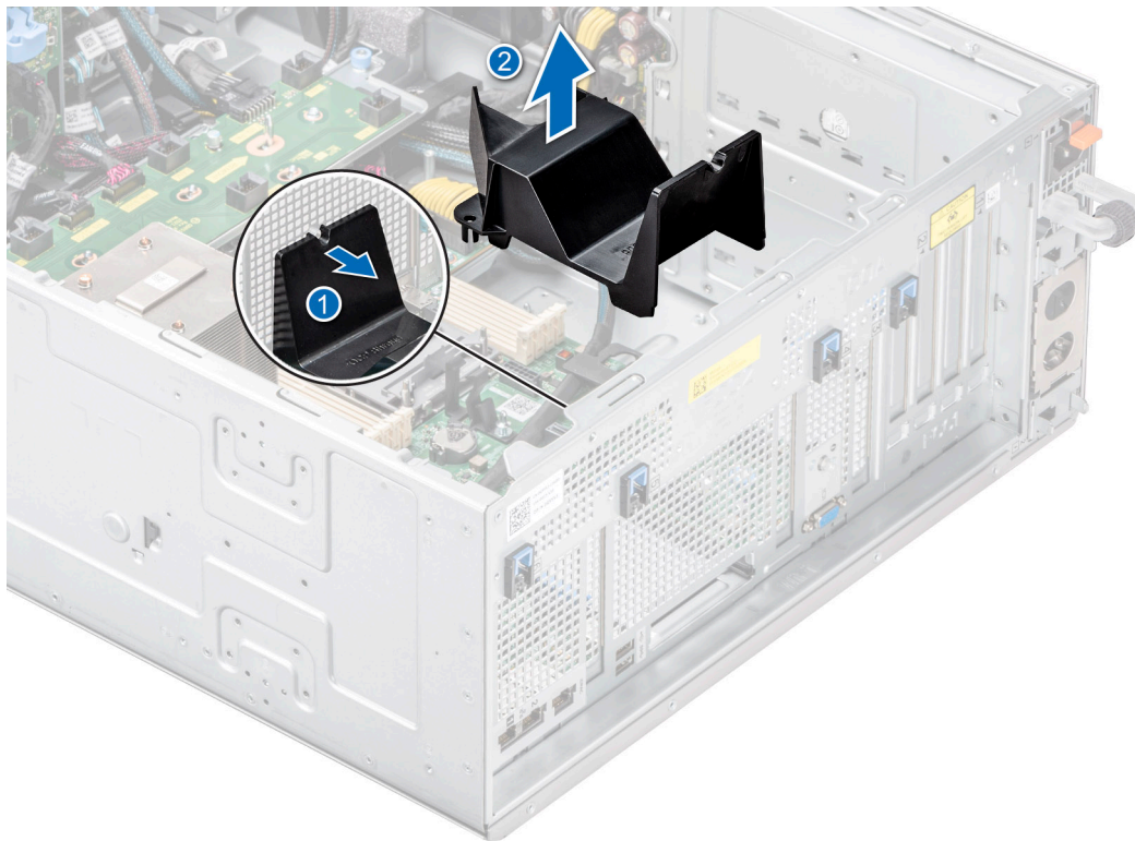
Figure 153. Removing the OCP air shroud
