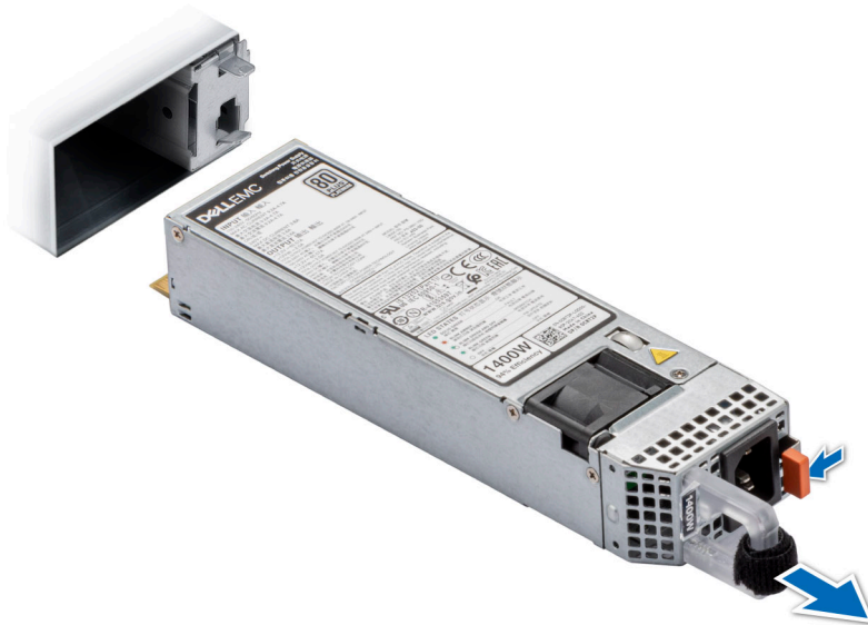
Figure 171. Removing a 60 mm power supply unit
