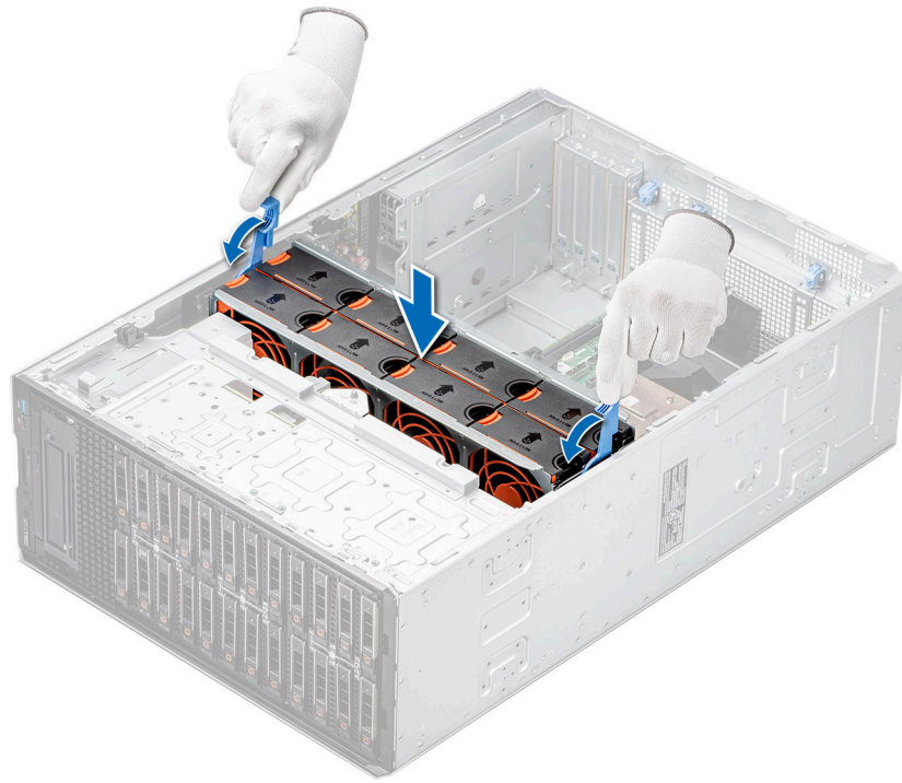
Figure 40. Installing the cooling fan cage
