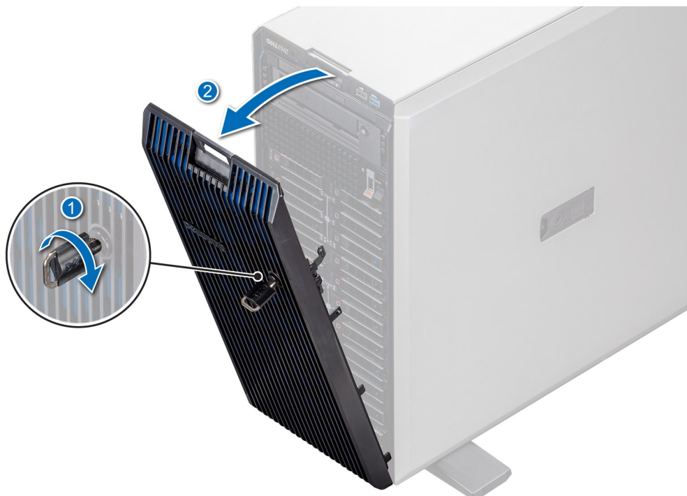
Figure 27. Removing the front bezel
