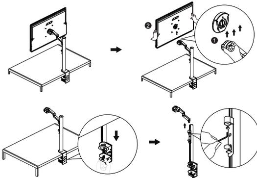
4. Remove the four screws and tripod from the rear cover to mount the monitor on the wall.
