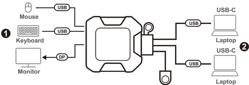
1. Connect the USB mouse, USB keyboard, and DisplayPort monitor into their respective ports on the US3312.
