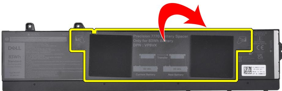
3. Flip the battery and peel the adhesive on the battery cable.
