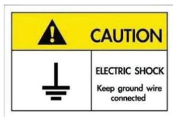
To avoid electric shock, the unit and its peripherals must be properly grounded (earthed).
