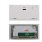
WP-580Txr is an extended range, HDBaseT wall plate transmitter for 4K@60Hz (4:2:0) HDMI signals over twisted pair. WP-580Txr inputs HDMI signals and converts them into an HDBaseT twisted pair signal that it transmits to a WP-580Rxr receiver. The WP-580Txr(D) model is supplied with a Midway Size 2 gang DECORA® design frame
