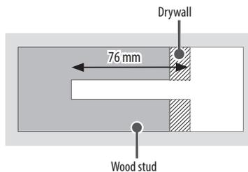
Use the  $\varnothing$  4 mm drill bit for wood to drill holes with the depth of 76 mm.
