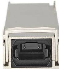
The QSFP40SR4ST is an MSA compliant fiber QSFP+ transceiver that's designed, programmed and tested to work with 40GBASE-SR4 compatible MSA switches and routers. The QSFP+ transceiver module supports a maximum distance of up to 150 m (492 ft) and delivers dependable 40 GbE connectivity over fiber cabling. **Technical Specifications:**
