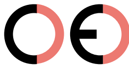
False CE Mark (too far)
