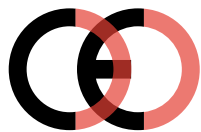
False CE Mark (too close)
