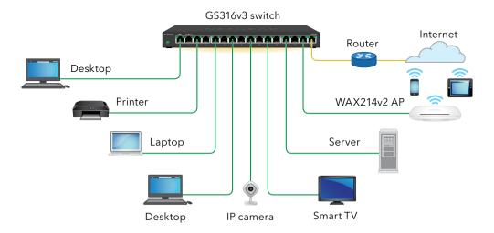
This switch is designed for indoor use only. If you want to connect it to a device located outdoors, the outdoor device must be properly grounded and surge protected, and you must install an Ethernet surge protector inline between the switch and the outdoor device. Failure to do so can damage the switch.
