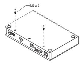
2. Use the screws from step 1 to attach the mounting bracket to the bottom of the transmitter, as shown below.
