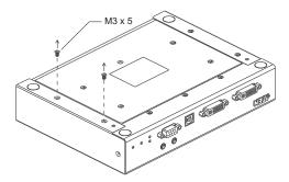
2. Use the screws from step 1 to attach the mounting bracket to the bottom of the transmitter, as shown below.
