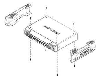
2. Remove the bottom and side screws from the unit.
