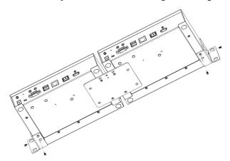
4. Screw the mounting brackets onto the rack.
