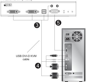
**Note:** The serial port on the transmitter (shown above) connects to the computer, while the serial port on the receiver (not shown) connects to a serial device (optional).
