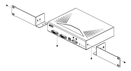
4. Screw the mounting brackets onto the rack.
