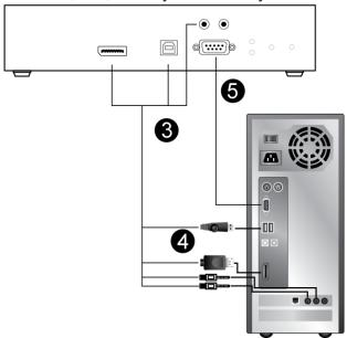
**Note:** The serial port on the Transmitter (shown above) connects to the computer; the serial port on the Receiver (not shown) connects to a serial device (optional).
