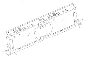
5. Screw the mounting brackets onto the rack.
