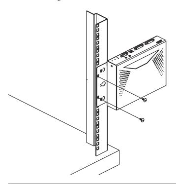
**Note:** Rack screws are not provided. We recommend the use of M5 x 12 Phillips Type I cross recessed screws.
