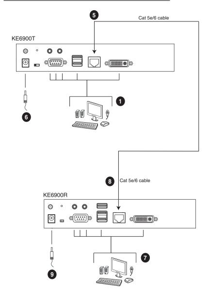
**Note:** The diagram above shows KE6900T and KE6900R. The KE6940 installation is the same except that an additional DVI monitor can be connected at each end for a dual-display setup.
