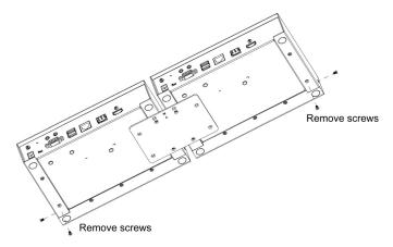
3. Use the screws in step 2 to install the left and right mounting brackets.
