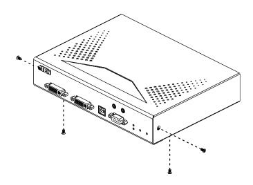
3. Use the screws in step 2 to install the right and left mounting brackets.
