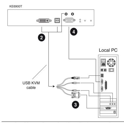
**Note:** The serial port on the transmitter (shown above) connects to the computer, while the serial port on the receiver (not shown) connects to a serial device (optional).
