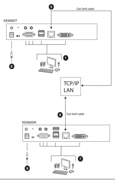
**Note:** The diagram above shows KE6900T and KE6900R. The KE6940 installation is the same except that an additional DVI monitor can be connected at each end for a dual-display setup.
