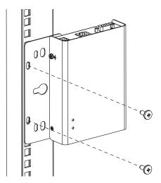
**Note:** Rack screws are not provided. We recommend the use of M5 x 12 Phillips Type I cross recessed screws.
