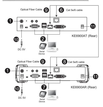
**Note:** The diagram above shows KE6900AT and KE6900AR. The KE6940A installation is the same except that an additional DVI monitor can be connected at each end for a dual-display setup.
