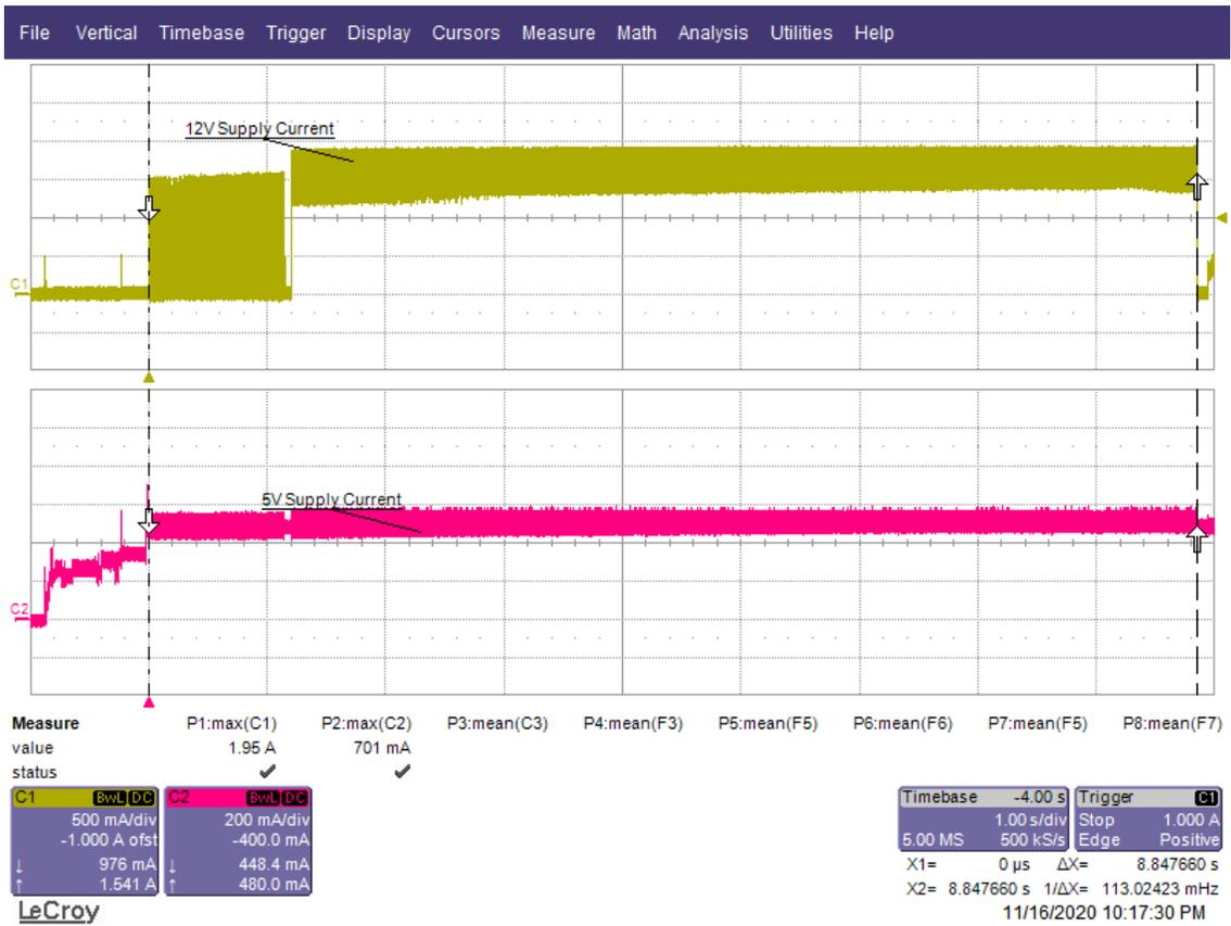
Figure 1. Typical 12V startup and operation current profile
