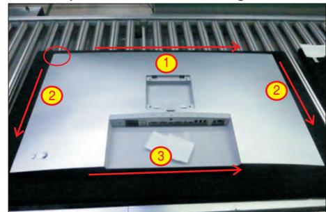
Lift the rear cover up carefully. Disconnect the joystick key cable from the connector of the interface board, and then remove the rear cover and put it aside for later disassembling.
