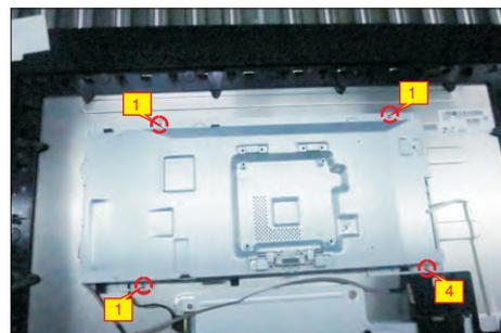
Lift up the middle bezel, and then put it on a cushion foam for later disassembling.
