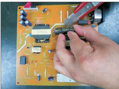
S21-4 Take out bulk cap. pin solder with soldering iron and absorber.
