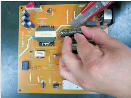
S21-3 Cut into the bottom of bulk cap. and pullit up carefully.
