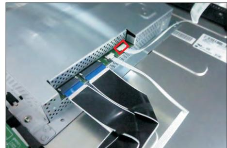
Use a Philips-head screwdriver to remove 2pcs screw for unlocking the key board, then tear off the tapes and release the key board.
