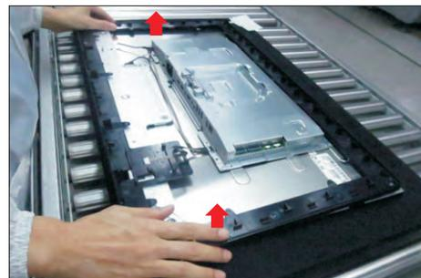
Tear off the tape on the middle bezel for releasing the LED cable, and then tear off the mylar tape to release the LED board for the hooks of the middle bezel.
