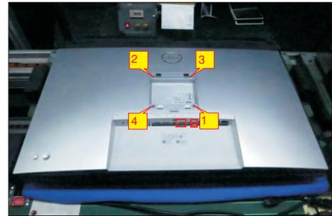
Tear off the screen protector, then wedge fingers between rear cover and the middle bezel on the corners of the top side of the monitor to release the rear cover, then use one hand to press the middle bezel, the other hand to pull up the rear cover in order of arrow preference for unlocking the rear cover.
