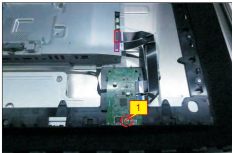
Use a Philips-head screwdriver to remove 18(13+5)pcs screws for unlocking the middle bezel with the panel module.
