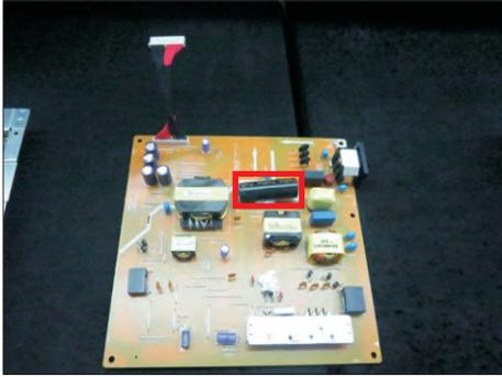
S21-1 Cut the glue between bulk cap. and PCB with a knife.
