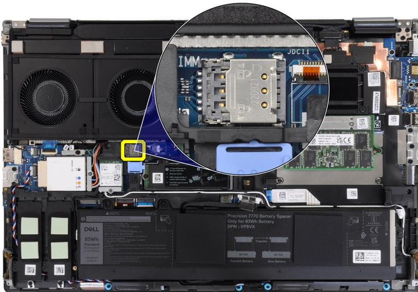
**CAUTION:** The SIM card cover is fragile and can be damaged if it is not properly unlocked before opening.
