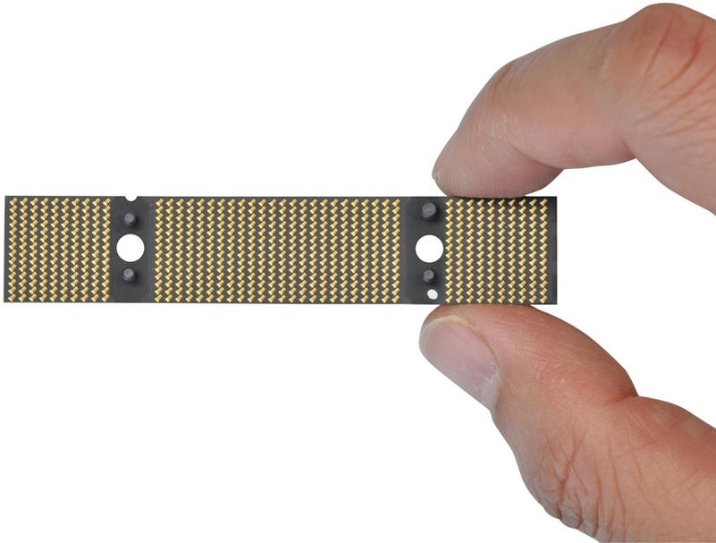
2. Place the memory interposer board on the system board.
