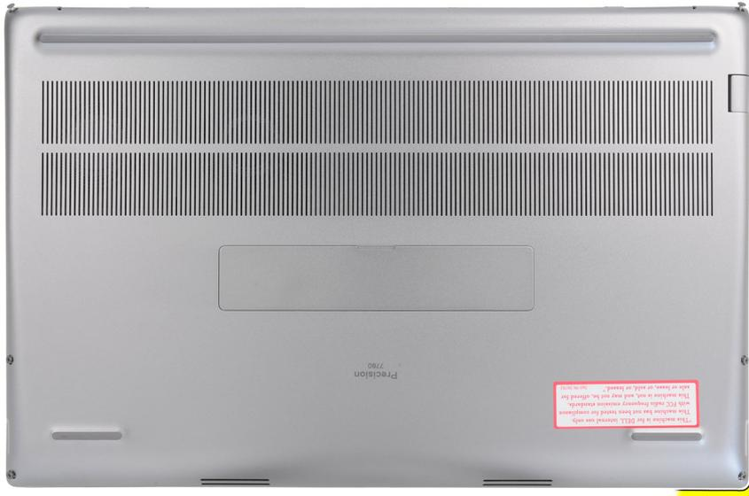
**NOTE:** For models shipped with smart-card reader, pry open the base cover from the smart-card reader slot at the bottom-right side of the base cover.
