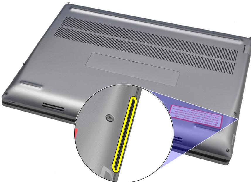
3. Lift the base cover starting from the bottom edge and push it towards the rear to remove it from the computer.
