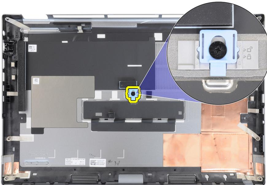
The door is unlocked by default. Push the latch downward to lock the door.
