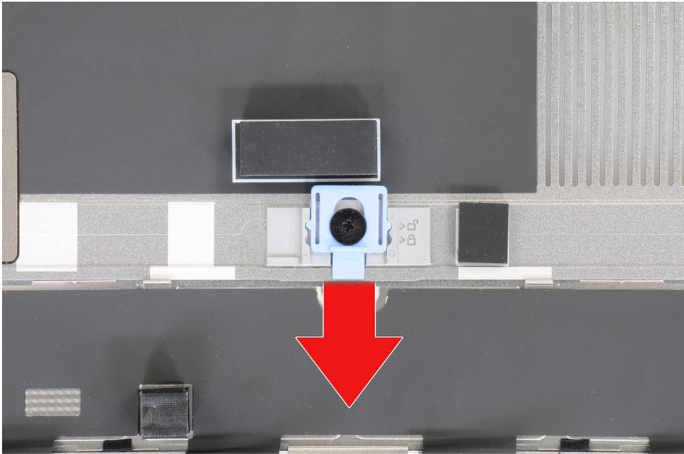
When the door is locked, push the latch upward to unlock the door.
