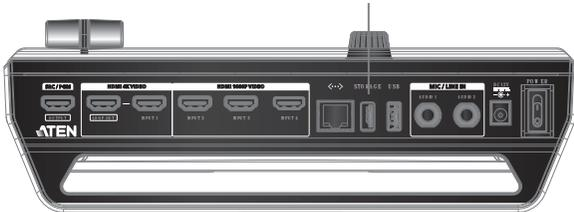
A warning message appears if there is no USB3.0 or later storage device plugged into the StreamLIVE™ PRO.
