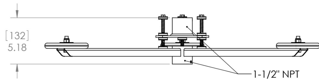
**UPPER AND LOWER PORTION CAN BE SEPARATED FOR EASE OF INSTALLATION**
