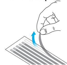
4. Carefully align the **Adhesive Strips** along the **Top, Bottom, Left, and Right** edges of the **Privacy Filter**. Apply **Firm Pressure** to affix them to the **Privacy Filter**.
