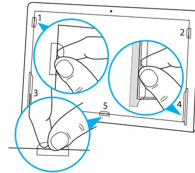
**Note** Depending on the display size, additional Mounting Tabs may need to be installed on the side or bottom bezels.
