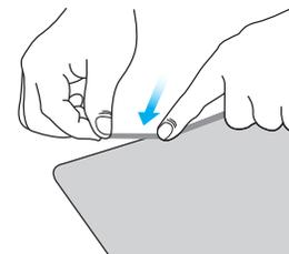
5. Carefully remove the **Protective Backing** from the **Adhesive Strips**
