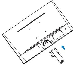
3. Hold the monitor base stand with both hands and firmly insert the base stand into the base column.
