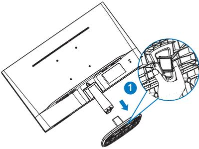
3. Press the release button to detach the base column.
