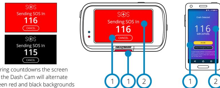
During countdowns the screen on the Dash Cam will alternate between red and black backgrounds to be as noticeable as possible.
