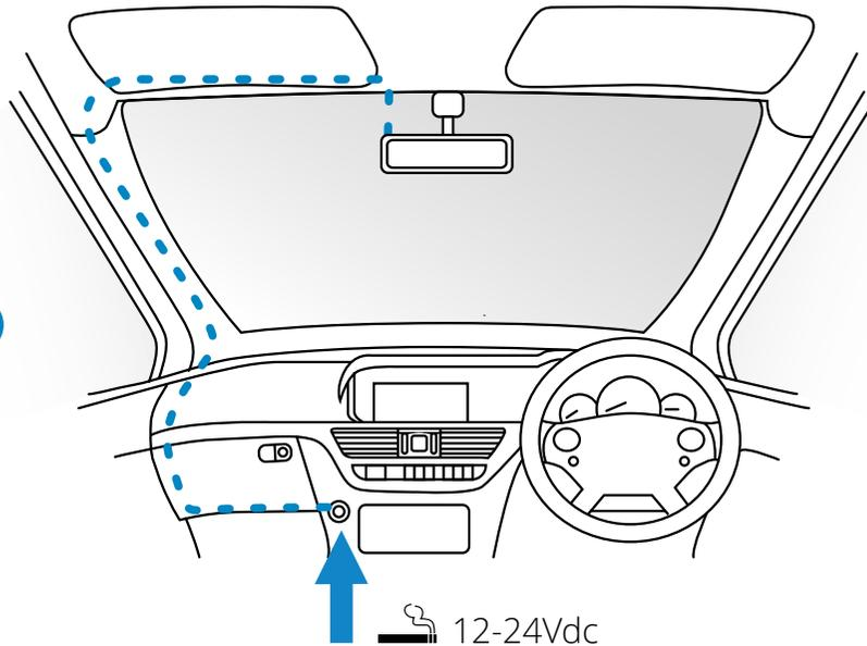
**5 Plug the power cable into the 12-24Vdc outlet of your vehicle**
