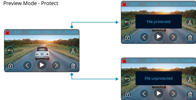
While in Preview Mode, press the Protect Button to protect/unprotect a file. When a file is protected, a red padlock icon will appear in the top left of the screen. You cannot protect or unprotect a video during playback.
