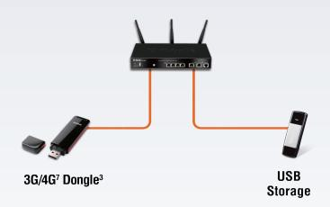
Supports one (DSR-150/150N/250/250N/500/500AC) or two (DSR-1000/1000AC) USB 2.0 devices to extend functionality.
