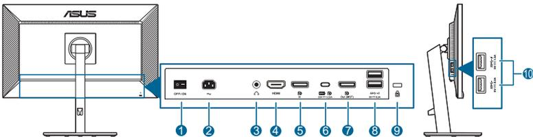
1. **Power switch.** Press the switch to turn on/off power.
