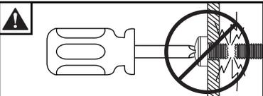
ENG Do not overtighten screws.
