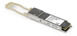
The JG325B-ST is an HPE JG325Bcompatible fiber transceiver module that has been designed, programmed and tested to work with HPE brand switches and routers. It delivers dependable 40 GbE connectivity over fiber cable, for 40GBASE-SR4 compliant networks, with a maximum distance of up to 150 m (492 ft).
