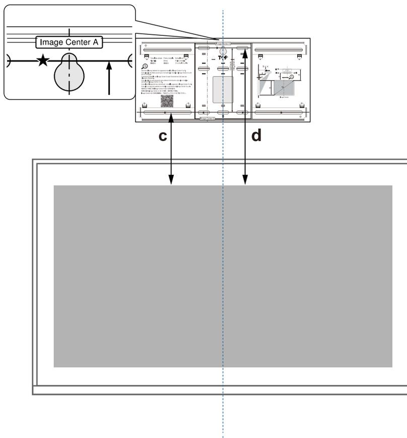
2 Drive a commercially available M10 screw into the position of the temporary screw hole for the wall plate
