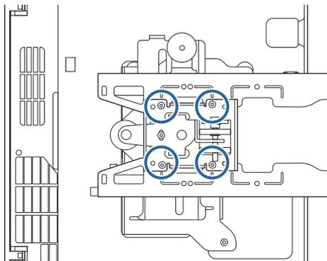
**2** Attach the adjustment unit to the setting plate with the M4 x 12 mm bolts (x4) supplied
