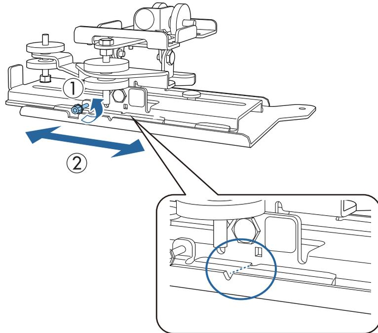
When the position is correct, tighten the M4 bolt.
