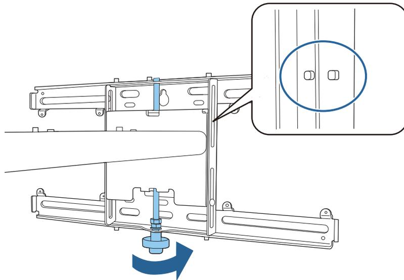
**7** Tighten the M6 bolt (x1) to secure the setting plate in position
