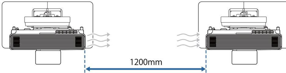
If you cannot secure a gap of approx. 1,200 mm, install a partition to block the heat vented from the projector's air exhaust vent.
