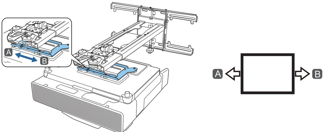
7 Loosen the M4 bolts (x2), and then adjust the forward/backward slide
