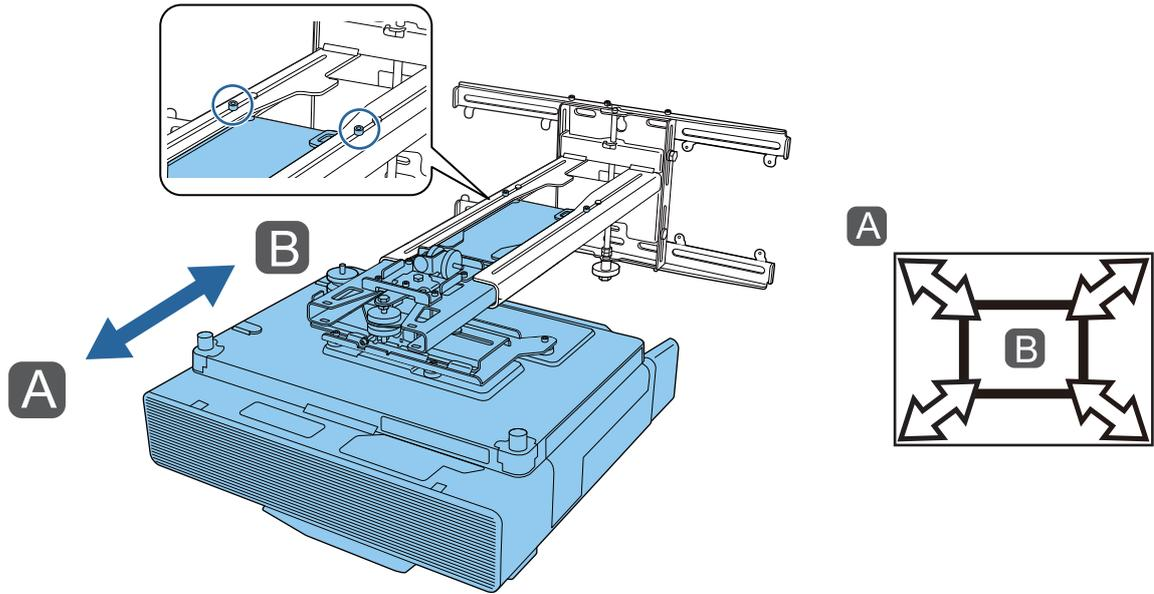
8 Loosen the M6 bolt, and then adjust the vertical slide
