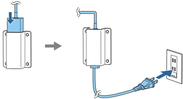
6 Connect the cable that is connected to the projector to the Control Pad
